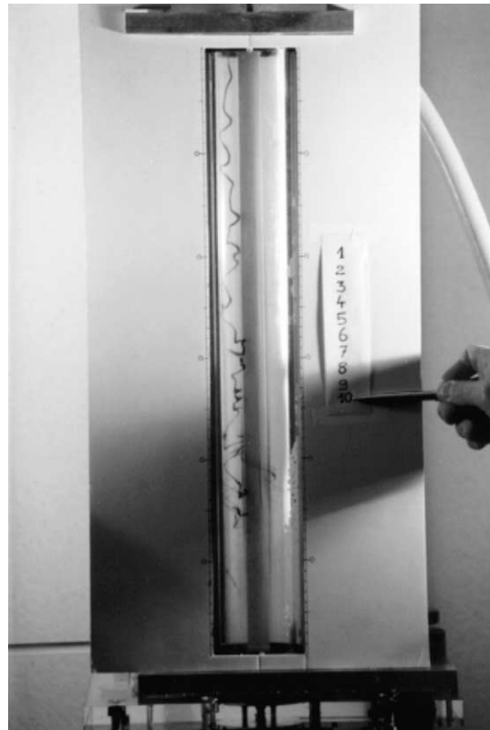
Fig. 5. Streaklines in the flow between confocal elliptic cylinders, the axial velocity is 1 mm/s.
